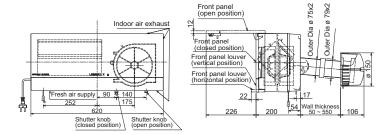
If the wall is thicker than 550mm, use the extension pipes and the pipe extension joints (separately sold parts).\*8
