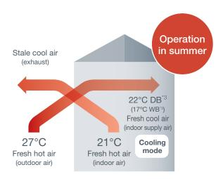
Lossnay's simultaneous air exhaust and supply provides balanced and effective ventilation allowing for a clean, fresh internal environment to be maintained in an energy efficient and cost effective manner.
